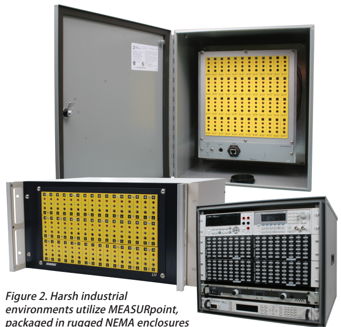
Figure 1. MEASURpoint incorporates proprietary ISO-Channel™ technology that makes measurements almost indestructible and eliminates any common mode noise and ground loop problems under all environmental conditions. In addition, up to forty-eight configurable input channels in groupings of eight voltage, thermocouple, and RTD inputs offer ultimate flexibility to the user.
