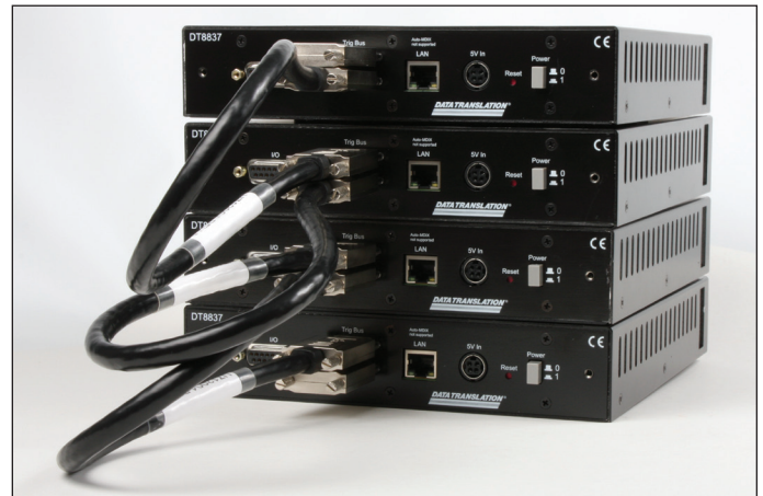
Figure 2. Up to sixteen modules may be used in parallel to connect a possible 64 direct voltage or IEPE channels, each synchronized in a master/slave configuration. The picture above shows four instrument modules in such a configuration. (See Figure 9).
