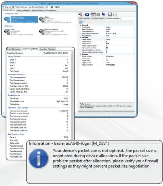
Matrox Capture Assistant GigE Vision and USB Vision <sup>3</sup> configuration and test tool
