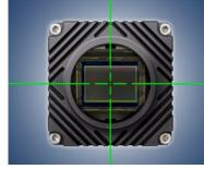
Active Sensor Alignment All Atlas cameras are actively aligned Sony Pregius sensors, up to 31 MP, to minimize sensor tilt and rotation, and to place the center of the sensor at the lens optical axis.
